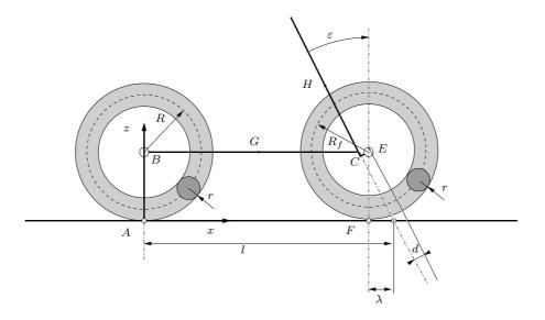
Figure 1: Geometry of the bicycle
