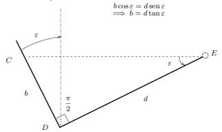
Figure 2: Geometry of the bicycle: the offset
